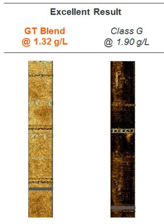
Figure 6: Results of wireline logging
