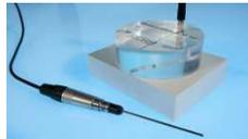
FES has recently increased its research capabilities with a brand new ASTM D5334-08 thermal conductivity measurement device. The heat transfer property of materials is of particular importance for geothermal energy. Together with existing temperature simulation software, the device expands the available technical expertise of which other industries can also profit. The measuring range is between 0,1 – 10 W/mK
